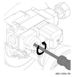
Fig. SUF 120-300 to 120-500 - CO<sub>2</sub> adjustment (partial load)
