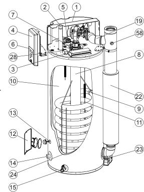
Fig. Water heater SUF 120-300, 120-400, 120-500
