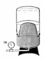
3. The pressure in the tank rises. Water continues to enter until the pump cut-out pressure is reached. The pump shuts off and the tank is now filled.
